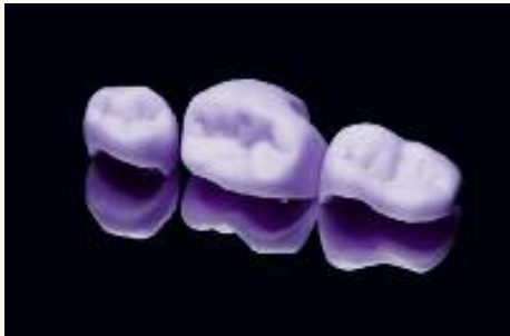
Fig. 8: Ground partial-coverage lithium disilicate crowns (e.max CAD LT, Ivoclar Vivadent) in their blue state prior to crystallisation firing.
